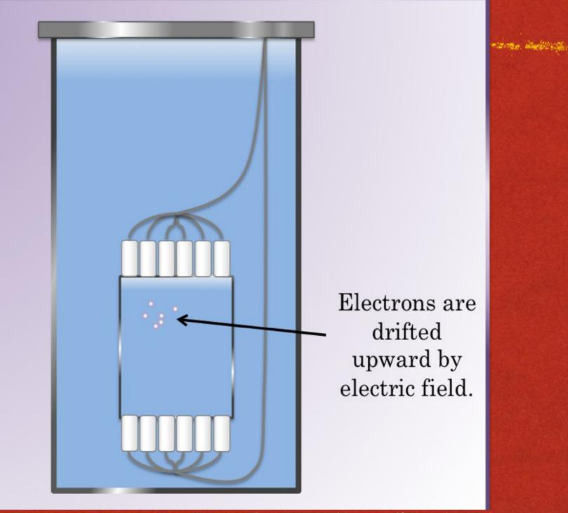
Electrons are extracted into gaseous argon, where the argon gas produces photons by electroluminescence. These photons are detected by the PMTs (s2).
